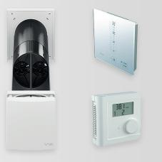
The Versus Duo decentralised heat recovery system is designed for ventilating a single room, making it ideal for bathrooms and kitchens. Designed for bathrooms and kitchens only, it is controlled via a wired controller and includes an integrated humidity sensor. Its thermal accumulator can recover up to 94% of the heat from the extracted air to warm the incoming air.
