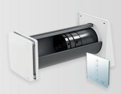
The Versus Silent decentralised heat recovery system can be installed individually or in pairs to ventilate specific areas of a home. Designed for living rooms, bedrooms, and offices, it is controlled via a wired controller and optional humidity sensors. Its thermal accumulator recovers up to 87% of the heat from extracted air to warm the incoming fresh air.
